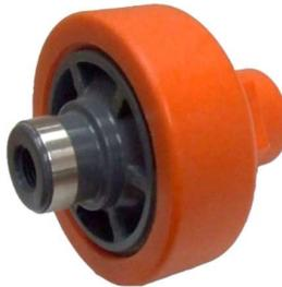
Polypropylene glass fibre reinforced top, EPDM diaphragm with PTFE coating on the process side, various bottom material available depending on the application, various process connections, maximum pressure 1000 kPa at 20°C for PVC-U & PP, at 40°C for PVDF.
