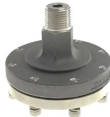
All stainless steel construction, ½" NPT female instrument connection and ½" NPT male process connection, (note: seal can be dismantled for cleaning without disturbing the calibration).
