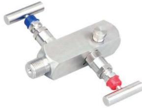
316 stainless steel construction, working pressure up to 40,000 kPa, 1/2" NPT female instrument connection and 1/2" NPT male process connection, 1/4" NPT vent/test port.
