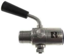
316 stainless steel construction, working pressure up to 10,000 kPa, 1/2" NPT female instrument connection and 1/2" NPT male process connection.
