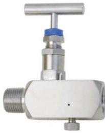
316 stainless steel construction, working pressure up to 40,000 kPa, 1/2" NPT female instrument connection and 1/2" NPT male process connection.
