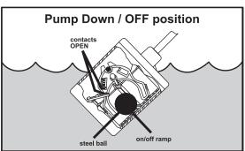
**Pump Down** is normally open contacts for emptying. **Pump Up** is normally closed contacts for filling. **SJE PumpMaster® SPDT** pump switch has 3 conductors for pump down and pump up operation.
