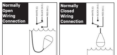
**Normally Open (High Level) Operation -** The float switch closes (turns on) when the switch tips slightly **above** horizontal signaling a high level, and opens (turns off) when the float switch drops slightly **below** horizontal in water or sewage applications.
