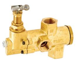
Details of construction include a forged brass body, brass and zinc-plated steel internal components, stainless steel springs, and glass filled fluropolymer poppets. Valve is available in two sizes, LGM20 for applications up to 20 SCFM, and LGM125 for applications up to 125 SCFM.
