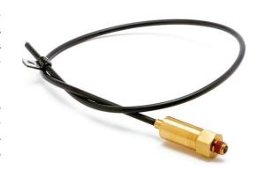
In operation, the vent unloader or pilot valve sends a pressure signal to the TC12 at the cut-out setting. This causes the TC12 piston to extend the control cable, which pushes the throttle lever, causing the engine to idle down. At the cut-in setting, the pressure signal going to the TC12 is vented, allowing the spring to return the piston, cable and throttle lever to the original full speed position.
