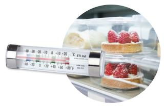
This spirit-filled fridge/freezer thermometer is encased in a clear ABS housing (20 x 30 x 122 mm). The thermometer's colour-coded zones indicate temperature over the range of -40 to 20 °C and -40 to 80 °F with a 1 °C resolution.
