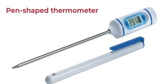
This pen-shaped thermometer measures temperature over the range of -49.9 to 149.9 °C, features a  $Ø3.5 \times 120$  mm stainless steel penetration probe and incorporates a °C/°F switch and display hold feature. Supplied with a probe cover that includes a pocket clip.
