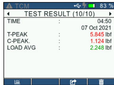
Saved results on the internal 32 GB SD card can be viewed and exported.
