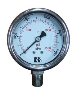
\* Formula:  $\pm 0.04$  x (t2 - t1) % of F.S. where t1 = reference temperature (+20°C) and t2 = ambient temperature in °C. Temperature Effect: The variation of indication caused by effects of temperature is to be calculated by the above formula; which is to be added to the specified accuracy during measurement. For higher process temperatures, please contact Ross Brown Sales.
